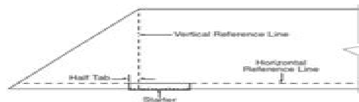
Figure 9-1: Starter strip overlapping the vertical reference line.
